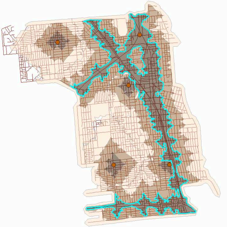
Figure 1. Map highlighting the unusually elongated (and inaccurate) service area of a fire station. The error is due to the accidental inclusion of railroad edges in the shapefile.
